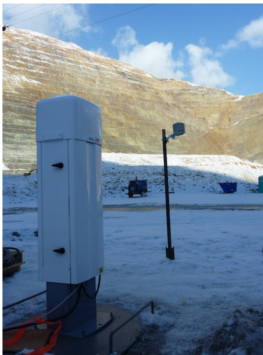
Figure 9. CL31 Ceilometer deployed in the Bingham Canyon Mine, with a temperature/humidity data logger in the background.
