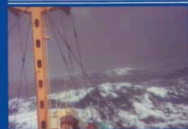
Force 11: Wind Speed 56-63 knots Sea: Wave height 11.5-16m (37-52 ft); Exceptionally high waves, sea covered with white foam patches, visibility still more reduced
