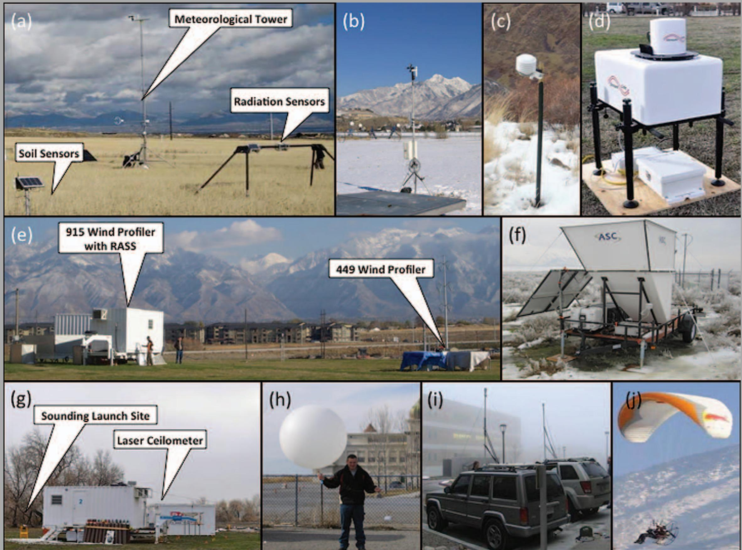
**FIG. 2. Photos of key PCAPS instrumentation. See Fig. 1 for location of instruments. (a) NCAR ISFS, (b) University of Utah automatic weather station, (c) University of Utah Hobo temperature dataloggers, (d) University of Utah scanning Doppler lidar, (e) and (g) NCAR ISS sites, (f) University of Utah minisodar, (h) University of Utah mobile radiosonde launch, (i) University of Utah mobile weather stations, and (j) instrumented motorized paraglider.**
