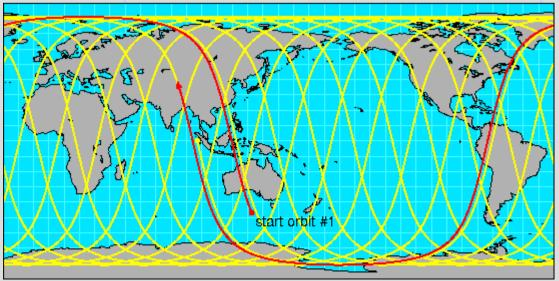
14 orbital tracks for a sun-synchronous satellite in near-polar orbit.: Daily coverage.
