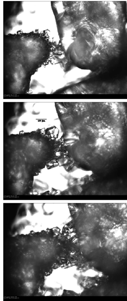
Fig. 2. At -15^{\circ}\text{C} , platelets are observed in this top-to-bottom time sequence. A connection is established between two grains. Also note that the branching on the lower left grain appears to develop around the crystal, indicating that the general vantage is likely onto the basal plane. a -axis plates are the dominant ice growth morphology at -15^{\circ}\text{C} . The time lapse between the first two images is 35 min and from the middle to the bottom is 1 hour 5 min. The image sequence was begun when a feature of interest was located.
