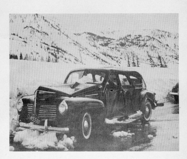
Damage to car by wet spring avalanche of moderate size.
