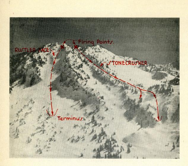
Controlled avalanches on Rustler Face and Stonecrusher. Note how Stonecrusher slide jumped over one gully and came down the next.
