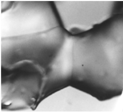
Figure 7. Snow grains stored at -24^{\circ}\text{F} for several years showing distinct grain-boundary grooves at the bonds.
