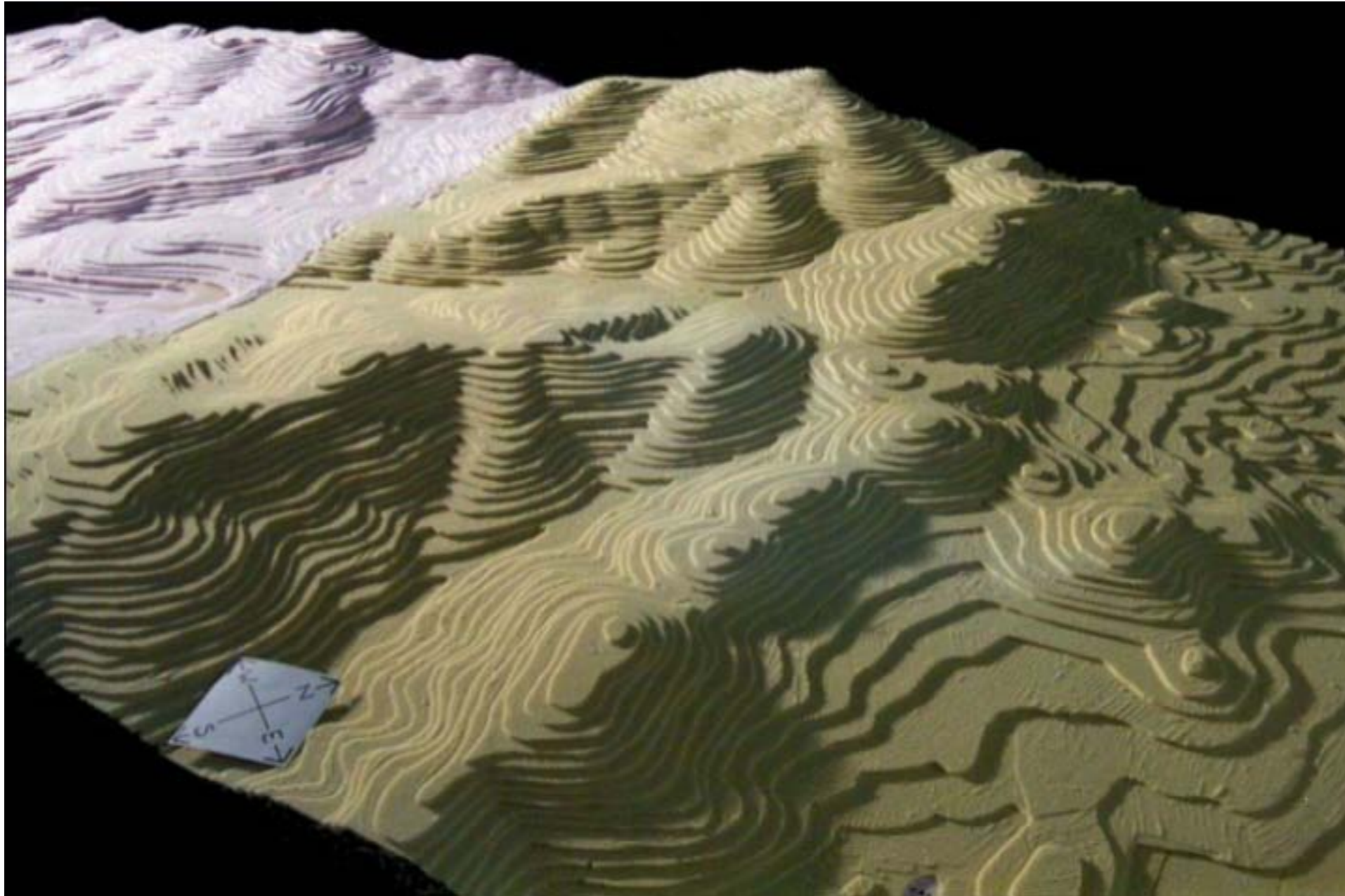
Figure 13-1 Scale model of Altamont Pass used in wind tunnel tests. (Source: Lubitz, W.D. and R.B White, “Prediction of Wind Power Production Using Wind-Tunnel Data, a Component of a Wind Power Forecasting System”
