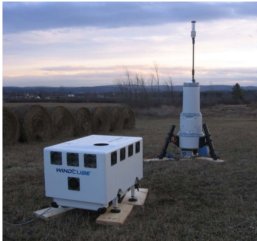
Figure 8-3 NRG/Leosphere's Windcube lidar (left) and Natural Power's ZephIR lidar unit. (Source: AWS Truepower)
