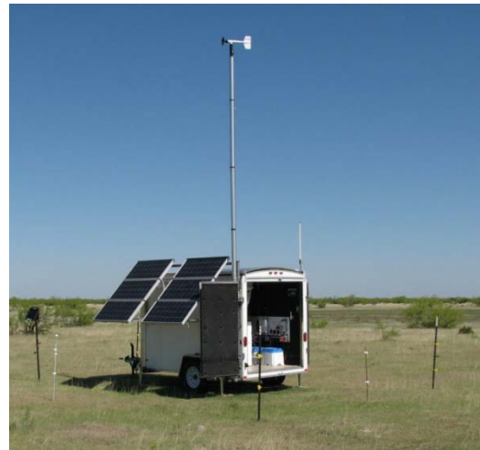
Figure 8-2 Left: Scintec SFAS sodar unit. Right: Atmospheric Research & Technology VT-1 sodar unit enclosed within a trailer. (Source: AWS Truepower)
