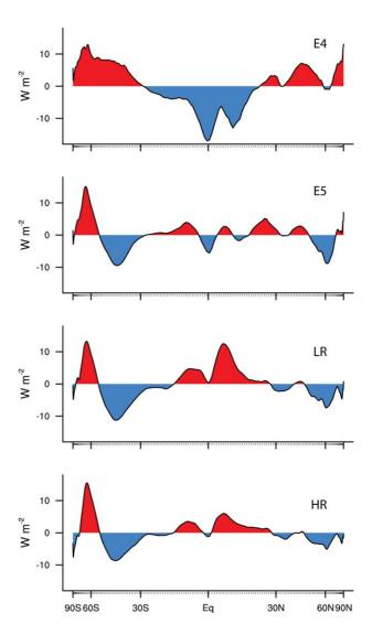
**Figure 4.** Differences between observed (CERES Ed2.6r) and simulated upward shortwave irradiance at TOA for three model generations (with two resolutions for ECHAM6). Fields are zonally and annually averaged and the mean bias is set to zero. Positive (red) regions indicate too much absorbed shortwave irradiance by the simulations.
