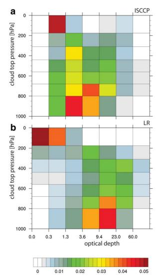
**Figure 6.** Cloud histogram showing the frequency of occurrence of cloudiness in optical thickness/cloud-top-pressure space for the period 1980–2005: (a) ISCCP; (b) LR-AMIP climatology based on the ISCCP simulator.
