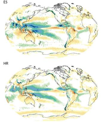
**Figure 7.** Difference in annual mean precipitation between ECHAM and GPCP (in units of mm  $d^{-1}$ ) for ECHAM5 (RMSE 1.35 mm  $d^{-1}$  upper), and the HR configuration of ECHAM6 (1.18 mm  $d^{-1}$  lower).
