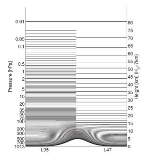
**Figure 1.** L47 and L95 hybrid vertical coordinate used in ECHAM6, shown here for the case of a 500 hPa surface pressure variation as might be associated with a large mountain.
