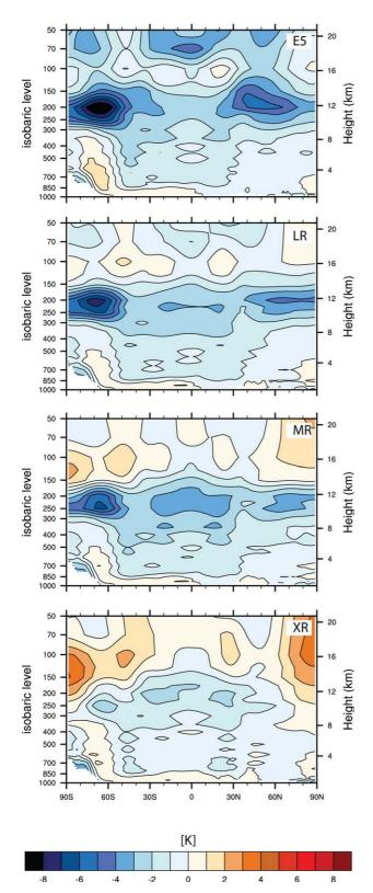
**Figure 12.** Differences between simulated and reanalysis (ERA-Interim) temperatures zonally averaged for the boreal winter (DJF) in the troposphere and lower stratosphere.
