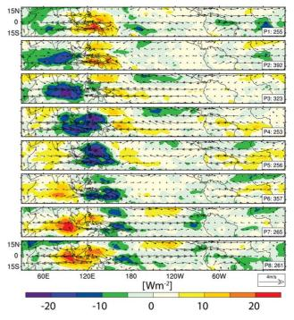
**Figure 9.** Madden Julian oscillation (MJO) lifecycle as represented in the MPI-ESM-HR. Nov-Apr 20–100-day filtered OLR (color) and 850 hPa wind anomalies regressed on the MJO index constructed from the square amplitude of the first two principle component time series derived from the multivariate EOF, following *Waliser et al.* [2009].
