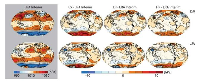
**Figure 14.** Mean sea-level pressure. (left) The climatology of the ERA-Interim is shown. (right) Differences relative to the reanalysis (ERA-Interim) for three different versions of ECHAM: ECHAM5, and the LR and HR configurations of ECHAM6.
