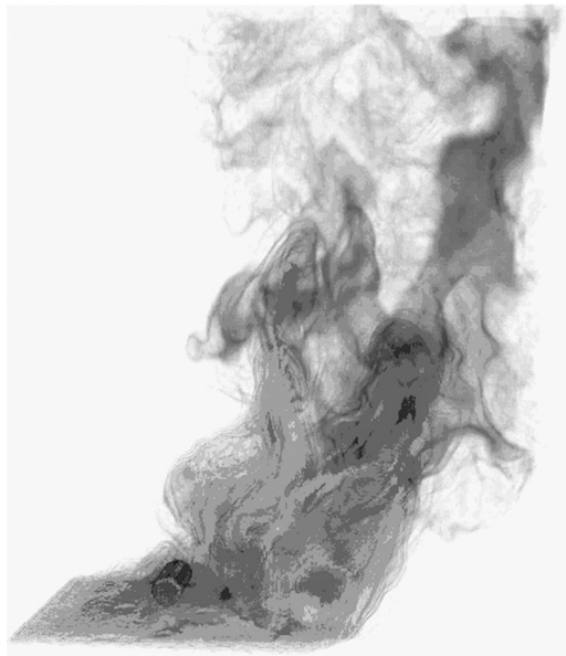
Figure 29: Volume-rendered image of the temperature field in the JP-8 pool fire with a 2.2 m/s crosswind. Side view showing region of highest temperature on upper leeward side of the container surface.
