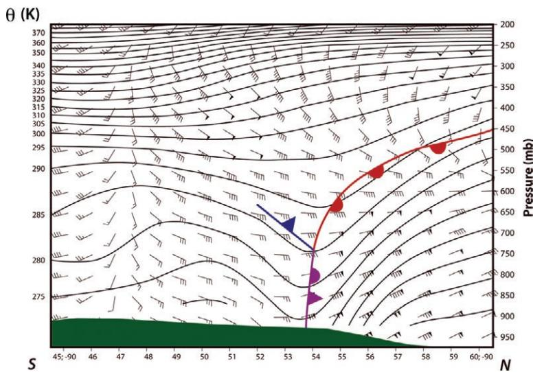
**FIG. 7.** North–south cross section through the warm-type occluded front in Fig. 6c. Potential temperature (solid lines every 5 K) and horizontal wind (pennant, full barb, and half-barb denote 25, 5, and 2.5 m s<sup>-1</sup>, respectively; separation between displayed wind vectors is 100 km). The ground is shown (green area), and the horizontal axis is labeled in degrees latitude.
