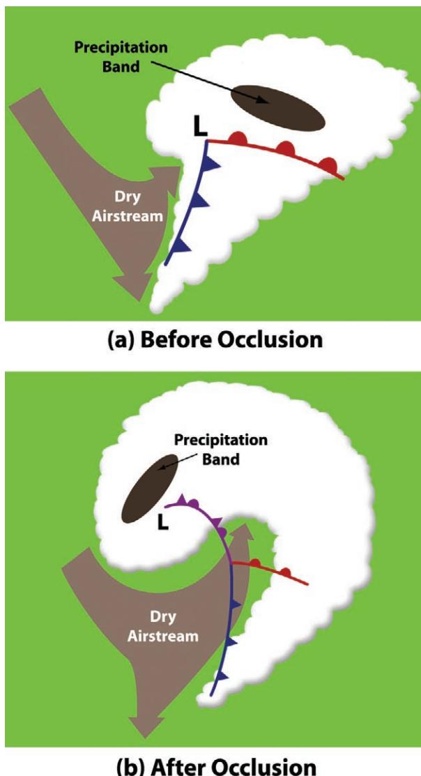
**FIG. 17. Schematic depiction of the evolution of the dry airstream, clouds, and regions where precipitation bands commonly occur (a) before and (b) after occlusion.**
