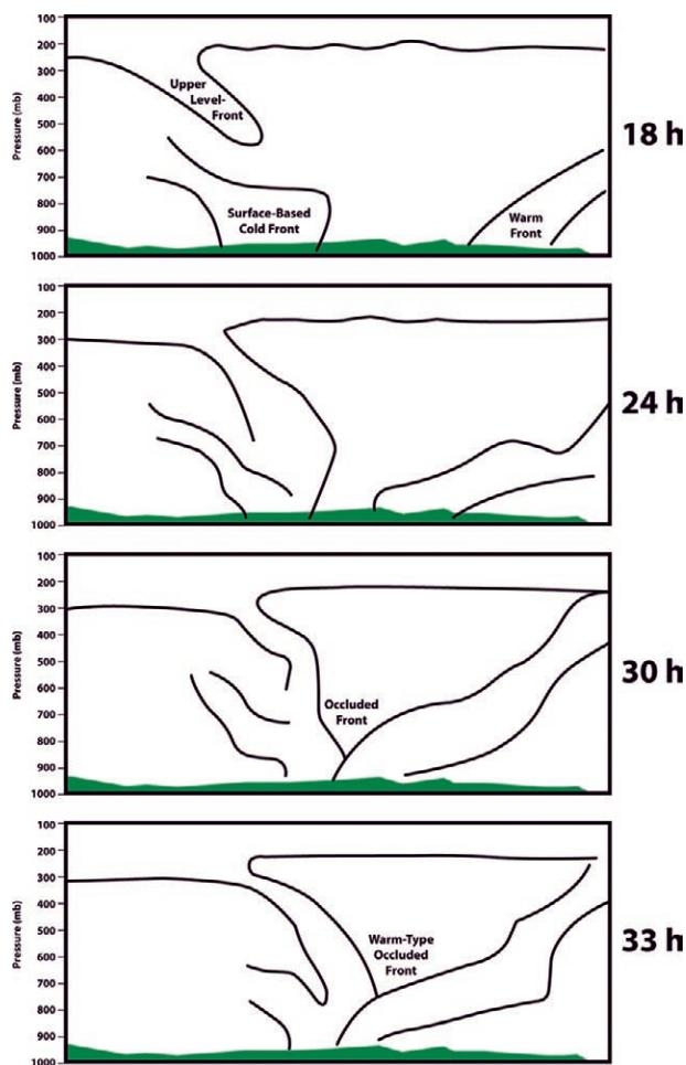
**FIG. 10.** Vertical cross sections of the formation of a warm-type occluded front at 18, 24, 30, and 33 h into a mesoscale model simulation initialized at 1200 UTC 14 Dec 1987. Heavy lines represent manually analyzed lines of temperature gradient discontinuities and the tropopause. The ground is shown (green area). [Caption and figure adapted from Fig. 9 in Schultz and Mass (1993).]
