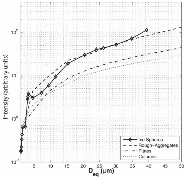
FIG. 4. Relationship between scattered intensity and area-equivalent spherical diameter in an FSSP-type probe for different idealized ice crystal particle shapes.
