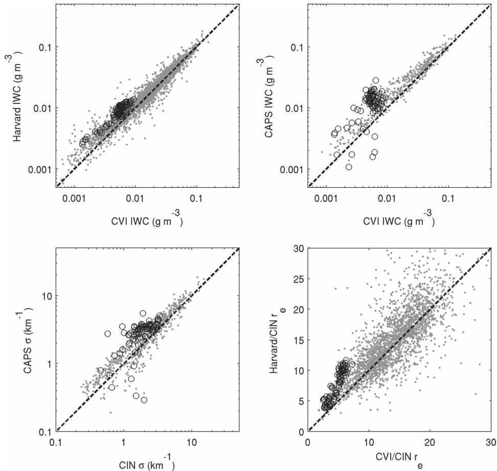
FIG. 5. Comparisons between instrument measurements of  $\sigma_{\text{ext}}$ , IWC, and  $r_e$  during MidCiX. The CAPS data represent a combination of the CAS and CIP instruments for particles between 2 and 1500  $\mu\text{m}$ . The Harvard water, CVI, and CIN probes are bulk instruments. Points in gray are from cirrus, and black circles are from wave clouds.
