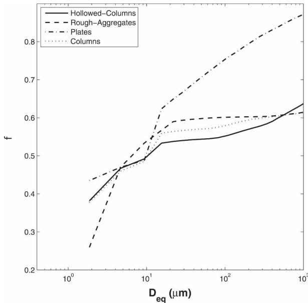
FIG. 3. Theoretical calculations of the fraction of scattering  $f$  not detected by the CIN, for various ice crystal shapes, as a function of area-equivalent spherical diameter. Here  $f$  is the integrated forward  $10^\circ$  of scattering by randomly oriented particles, according to phase-function data described by Yang and Liou (1998).
