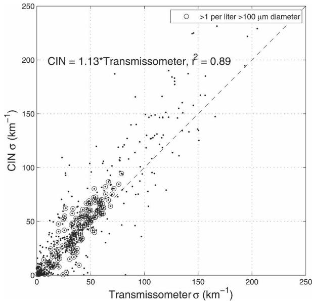
FIG. 6. Comparison of the CIN extinction coefficient  $\sigma$  with the Nevzorov transmissometer  $\sigma$  in warm cumulus during ICARTT. Circles indicate time periods when the concentration of particles  $>100 \mu\text{m}$  diameter was greater than  $1 \text{ L}^{-1}$  (maximum measured was  $26 \text{ L}^{-1}$ ).
