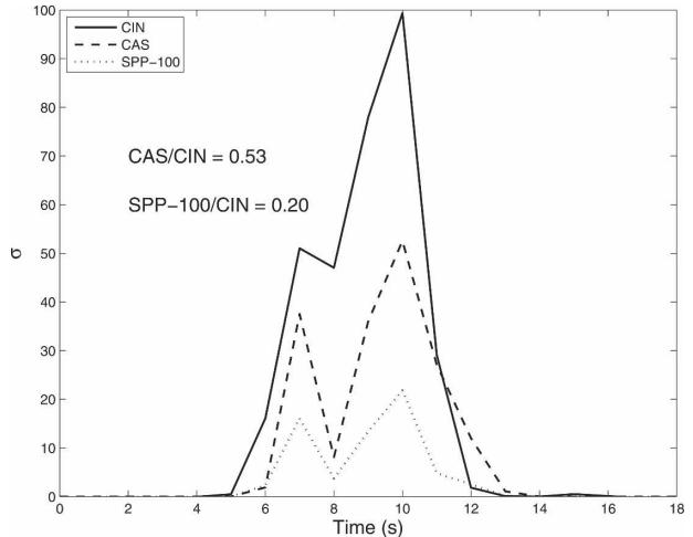
FIG. 2. Measured values of the extinction coefficient  $\sigma$  taken with CAS, SPP-100, and CIN probes flown by the WB-57F aircraft in trade wind cumulus near Key West between 85 581 and 85 524 s UTC on 28 Jul.
