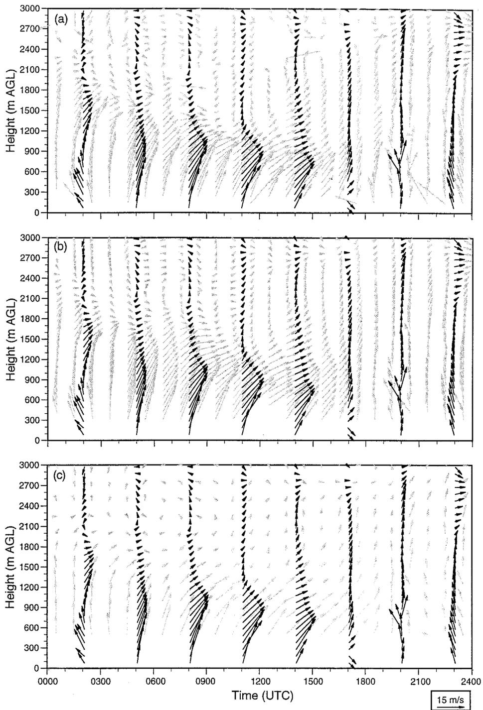
FIG. 7. Comparison of rawinsonde vector wind profiles (dark vectors), averaged over 100-m height intervals, with those measured (gray vectors) by (a) the low mode of the 915-MHz wind profiler, (b) the high mode of the 915-MHz wind profiler, and (c) the 404-MHz wind profiler for a 24-h period starting at 1800 CST 31 July 1994.
