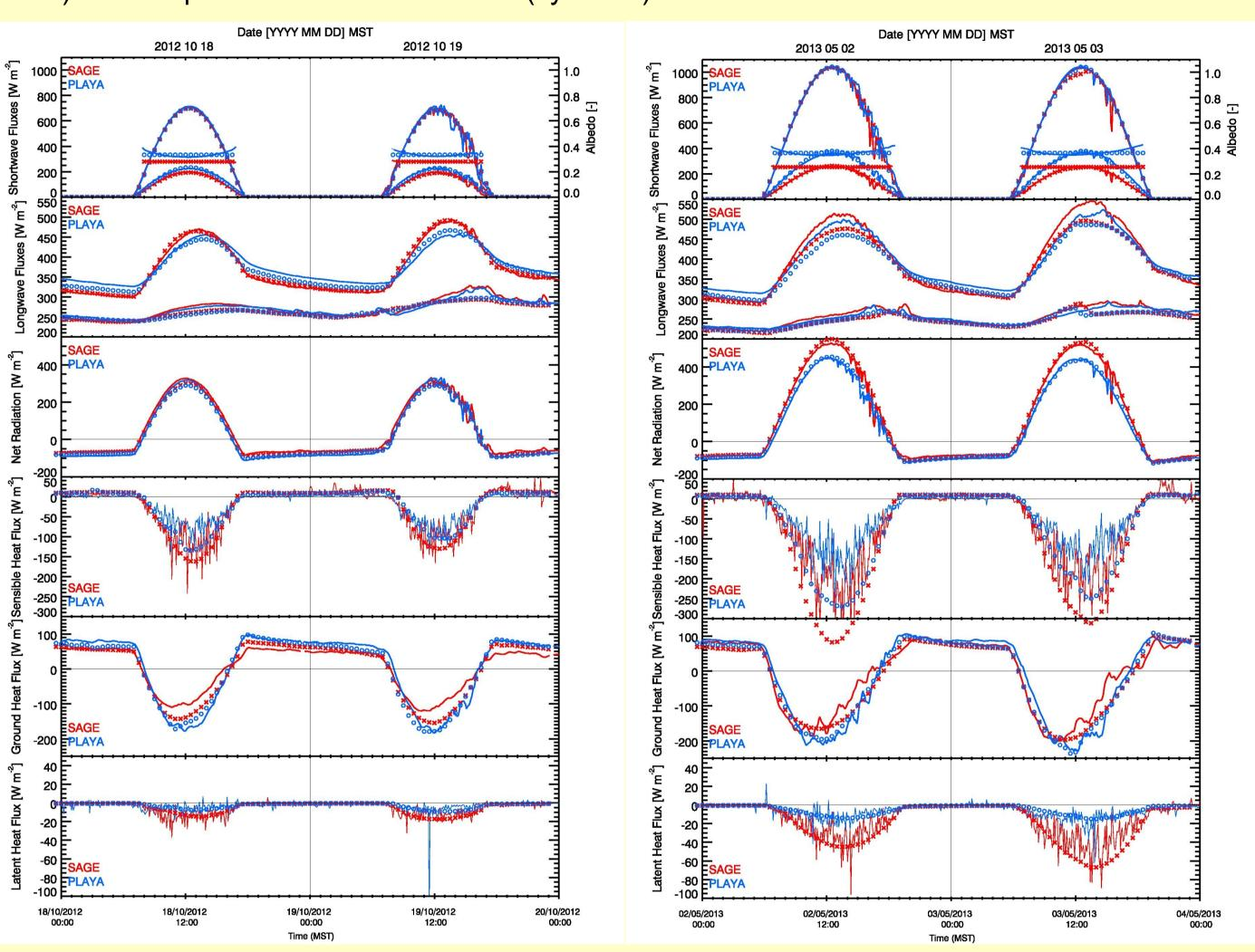
c) Budget residual While the energy balance is closed at nighttime, a large residual term is found during the day. Residuals of similar magnitude have been observed in many field campaigns. The cause for these residuals is still unknown. Comparisons with the WRF simulation points to an underestimation of the sensible heat flux.
