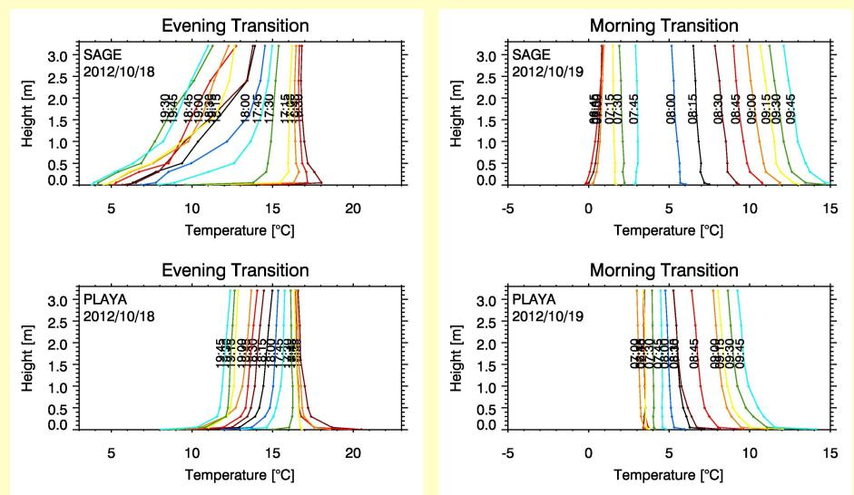
The Playa soil with its higher thermal conductivity takes up and releases more energy then the soil at the Sagebrush site. The release of this stored heat at Playa leads to a less rapid cooling of the near-surface air in the evening. In the morning, the heat uptake leads to less rapid near-surface heating.
