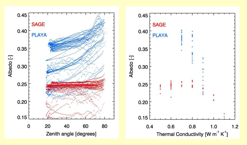
a) Albedo differences between the Playa and Sagebrush sites highlight the role of specular reflection. Soil moisture observations failed due to highly saline soils, but thermal conductivity variations indicate soil moisture effects on albedo.
