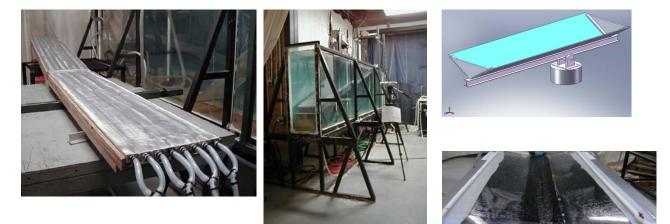
**FIGURE 15a:** Experiments on katabatic and anabatic flows with slope discontinuities. The slopes can be heated or cooled by circulating water via a series of internal passages that help distribute the heat flux uniformly.
