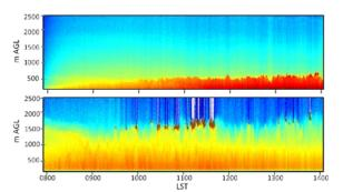
**FIGURE 11:** UV Aerosol Lidar (Leosphere ALS300) images (staring mode) on two different days. Range Height Indicator (RHI) scans will be performed using elevation ranges from 2 degrees to 90 degrees to provide details on cloud cover, CBL height and aerosol layer structure.
