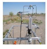
**FIGURE 9:** The sonic-Hot-film combo (Kit et al. 2010) will probe down to Kolmogorov scale of turbulent kinetic energy dissipation.
