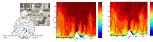
**FIGURE 13:** Exploratory RF polarimetric sensing test. Note the changes in clutter response due to land surface water.
