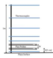
**FIGURE 8:** A schematic illustrating the placement of the near-surface flux probes within a dense array of thermocouples.
