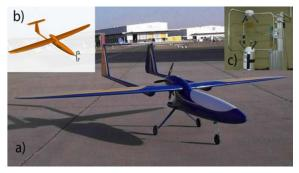
**FIGURE 12:** (a) Silvertone Flamingo Mark 4 UAV (length 2m; wingspan 4m; Moki 180 gas engine, 5.6 liter fuel tank; payload 15 lbs; 30-90 mph); (b) instrument mounting plan developed in consultation with the manufacturer; (c) on-going UAV instrument development at ND (www.flamingouav.com); see §3.3.2.
