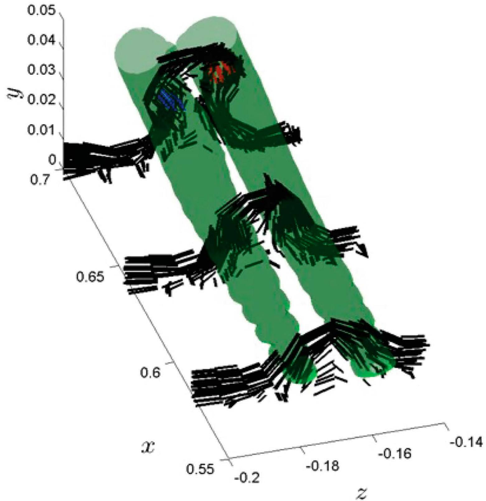
**A pair of counterrotating, coherent (and vortical) structures (green isosurfaces) and accompanying vortex filaments (black)**
