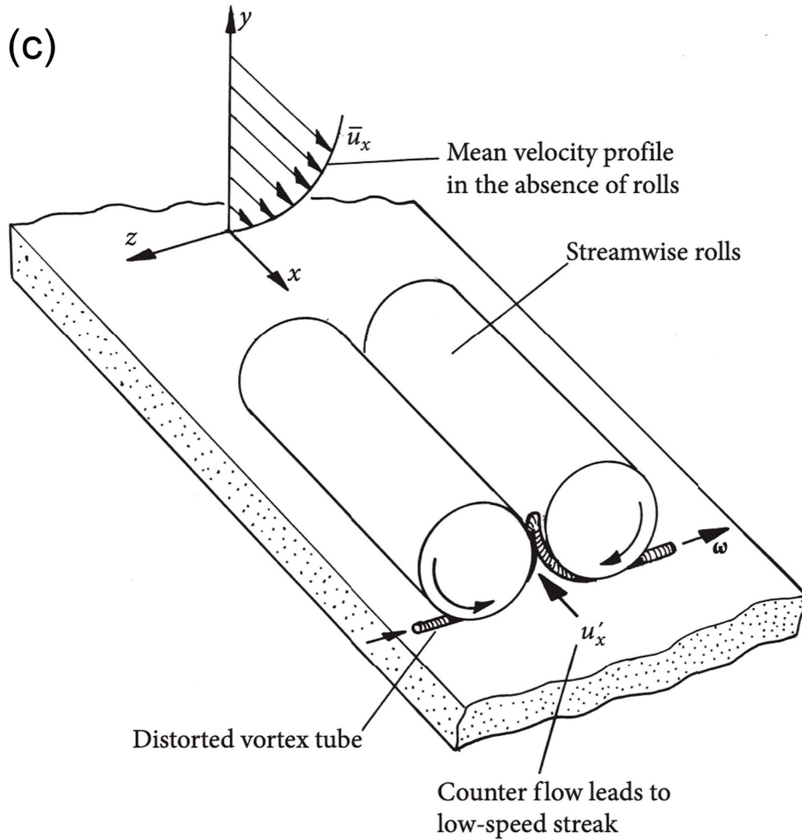
**Coherent structures in the surface layer with an attendant vortex line.**
