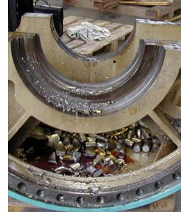
Premature fatigue of a turbine's main shaft bearing, courtesy S. Schreck, NREL
