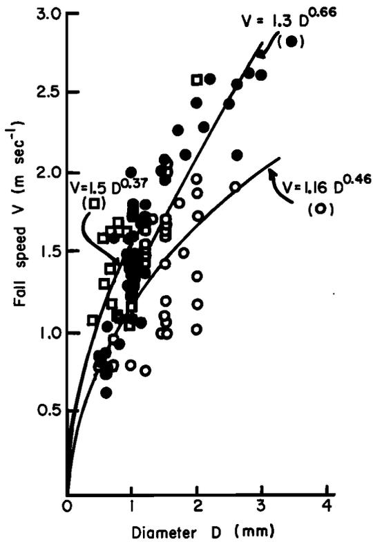
Fig. 5. Fall speeds versus diameters for lump graupel of three different density ranges: open circles, 0.05–0.1 Mg m<sup>-3</sup>; solid circles, 0.1–0.2 Mg m<sup>-3</sup>; and squares, 0.2–0.45 Mg m<sup>-3</sup>.
