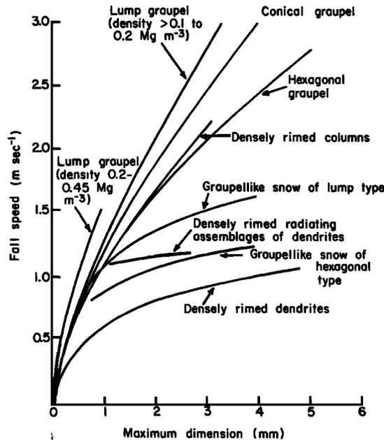
Fig. 17. Best-fit lines for fall speeds versus maximum dimensions of single solid precipitation particles of various types.
