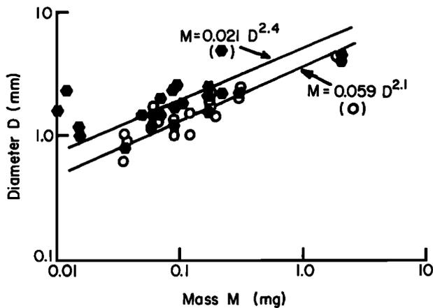
Fig. 11. Diameters versus masses for graupellike snow of lump type (circles) and hexagonal type (hexagons).
