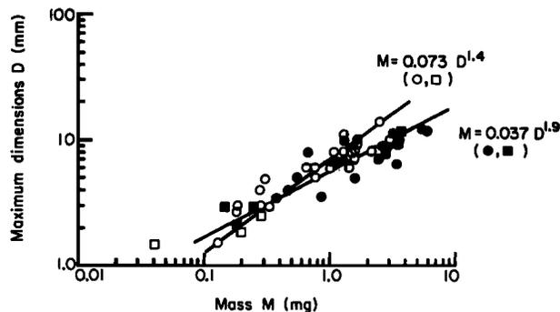
Fig. 21. Maximum dimensions versus masses for unrimed aggregates of radiating assemblages of dendrites (open circles), densely rimed aggregates of radiating assemblages of dendrites (solid circles), unrimed aggregates of dendrites (open squares), and densely rimed aggregates of dendrites (solid squares).
