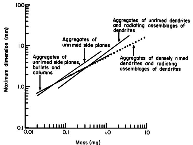
Fig. 25. Best-fit curves for maximum dimensions versus masses of aggregates of various types.
