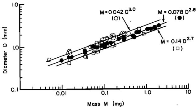
Fig. 6. Diameters versus masses for lump graupel of three different density ranges: open circles, 0.05–0.1 Mg m<sup>-3</sup>; solid circles, 0.1–0.2 Mg m<sup>-3</sup>; and squares, 0.2–0.45 Mg m<sup>-3</sup>.
