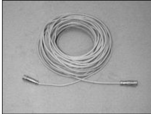
Figure 5 Cable between Junction Box and RCPD
