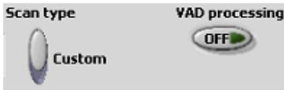
With the custom file, the option is available to perform **VAD processing** on the data. This processing option will only work on single elevation, arc scanning configurations where the arc covers 90 degrees or more in azimuth.
