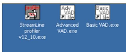
The Advanced VAD and Basic VAD modules are used to set up VAD scans for use with the main ‘StreamLine Profiler’ software.
