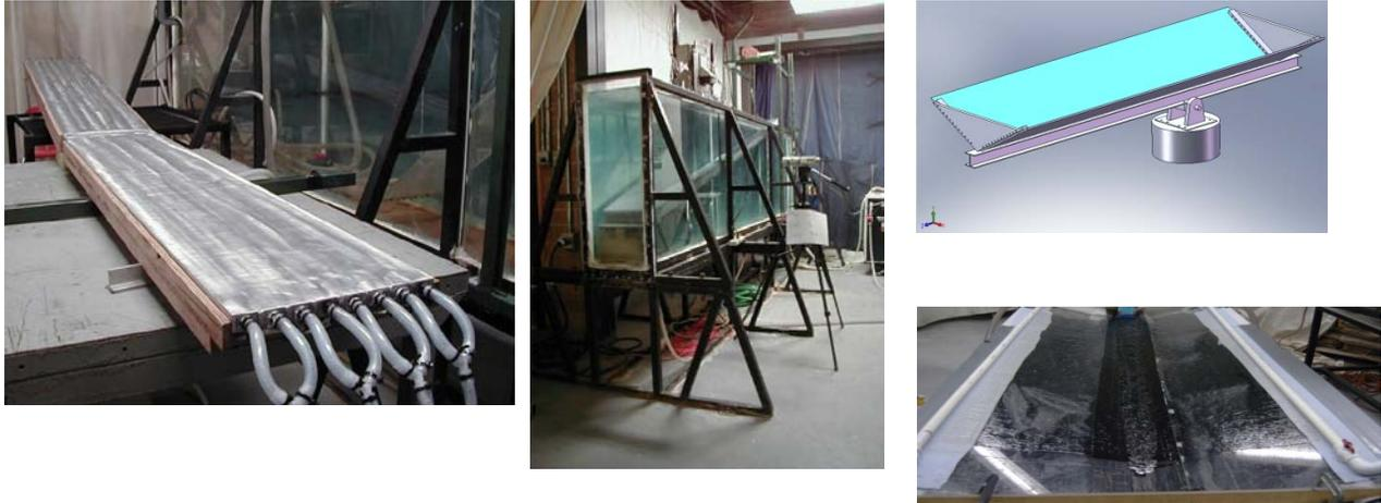
**FIGURE 15a:** Experiments on katabatic and anabatic flows with slope discontinuities. The slopes can be heated or cooled by circulating water via a series of internal passages that help distribute the heat flux uniformly.
