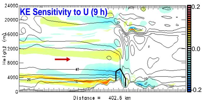
**FIGURE 5:** An example of a COAMPS adjoint sensitivity calculation for wind normal to the Sierra. The COAMPS adjoint was integrated over a nine hour period to compute the sensitivity of a kinetic energy response function (within the bold black outline) to the cross-barrier (U) wind component.
