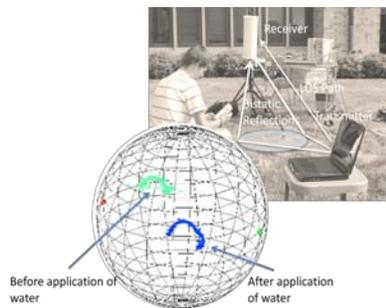
**FIGURE 13:** Exploratory RF polarimetric sensing test. Note the changes in clutter response due to land surface water.
