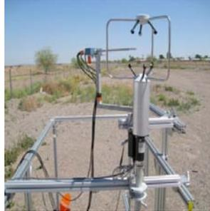
**FIGURE 9:** The sonic-Hot-film combo (Kit et al. 2010) will probe down to Kolmogorov scale of turbulent kinetic energy dissipation.
