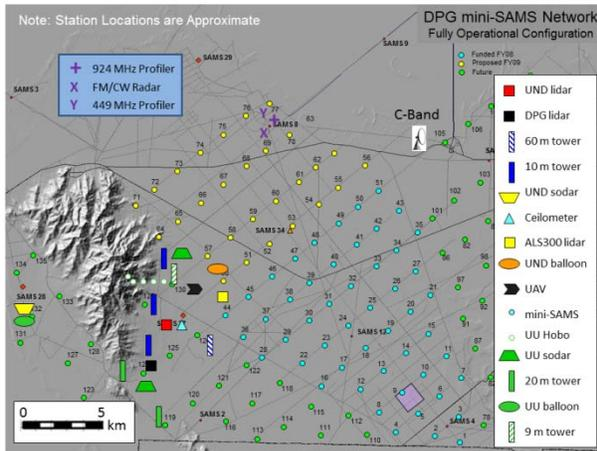
**FIGURE 6:** The GMAST and placement of selected instrumentation (tentative). Doppler and ALS 300 Lidars will be relocated, as needed.
