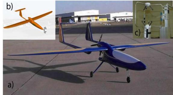
**FIGURE 12:** (a) Silverstone Flamingo Mark 4 UAV (length 2m; wingspan 4m; Moki 180 gas engine, 5.6 liter fuel tank; payload 15 lbs; 30-90 mph); (b) instrument mounting plan developed in consultation with the manufacturer; (c) on-going UAV instrument development at ND ([www.flamingouav.com](http://www.flamingouav.com)); see §3.3.2.
