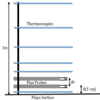
**FIGURE 8:** A schematic illustrating the placement of the near-surface flux probes within a dense array of thermocouples.
