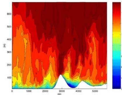
**FIGURE 14a:** Streamwise velocity over Askervein Hill; computations were conducted using TKE-1.5 closure.
