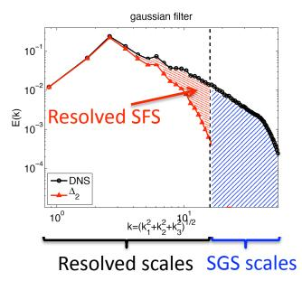
The Gaussian filter (or box filter) does not have as compact of support in wavespace as the cutoff filter. This results in attenuation of energy at scales larger than the filter scale. The scales affected by this attenuation are referred to as **Resolved SFSs**.
